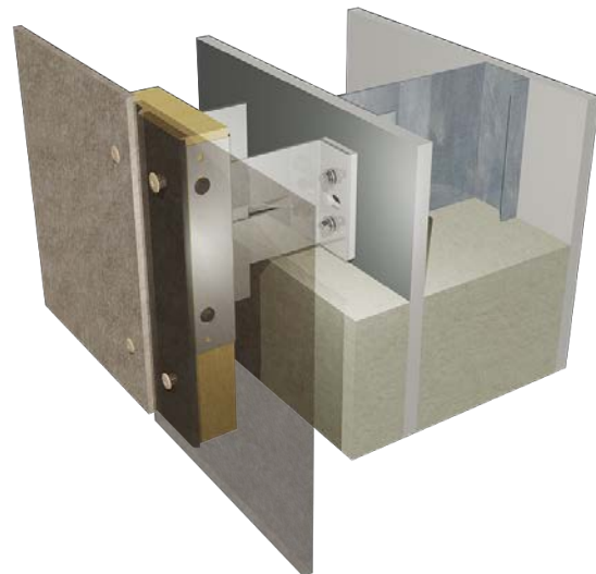
Visible Fixing (Screws to Timber battens)
